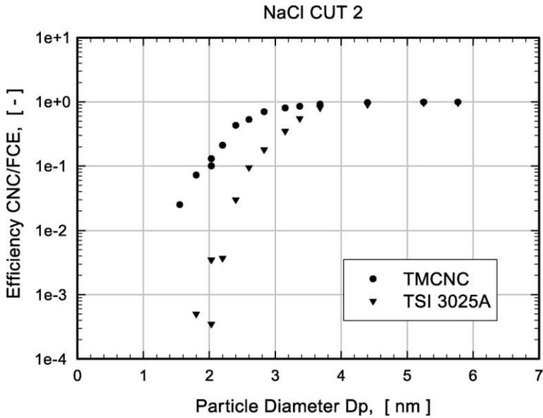
Fig. 4. Experiment NaCl CUT 2: response characteristics of the readjusted TM CNC and the TSI 3025A for monodispersed NaCl test aerosols, geometric mean particle diameters between 1.5 and 6 nm.
