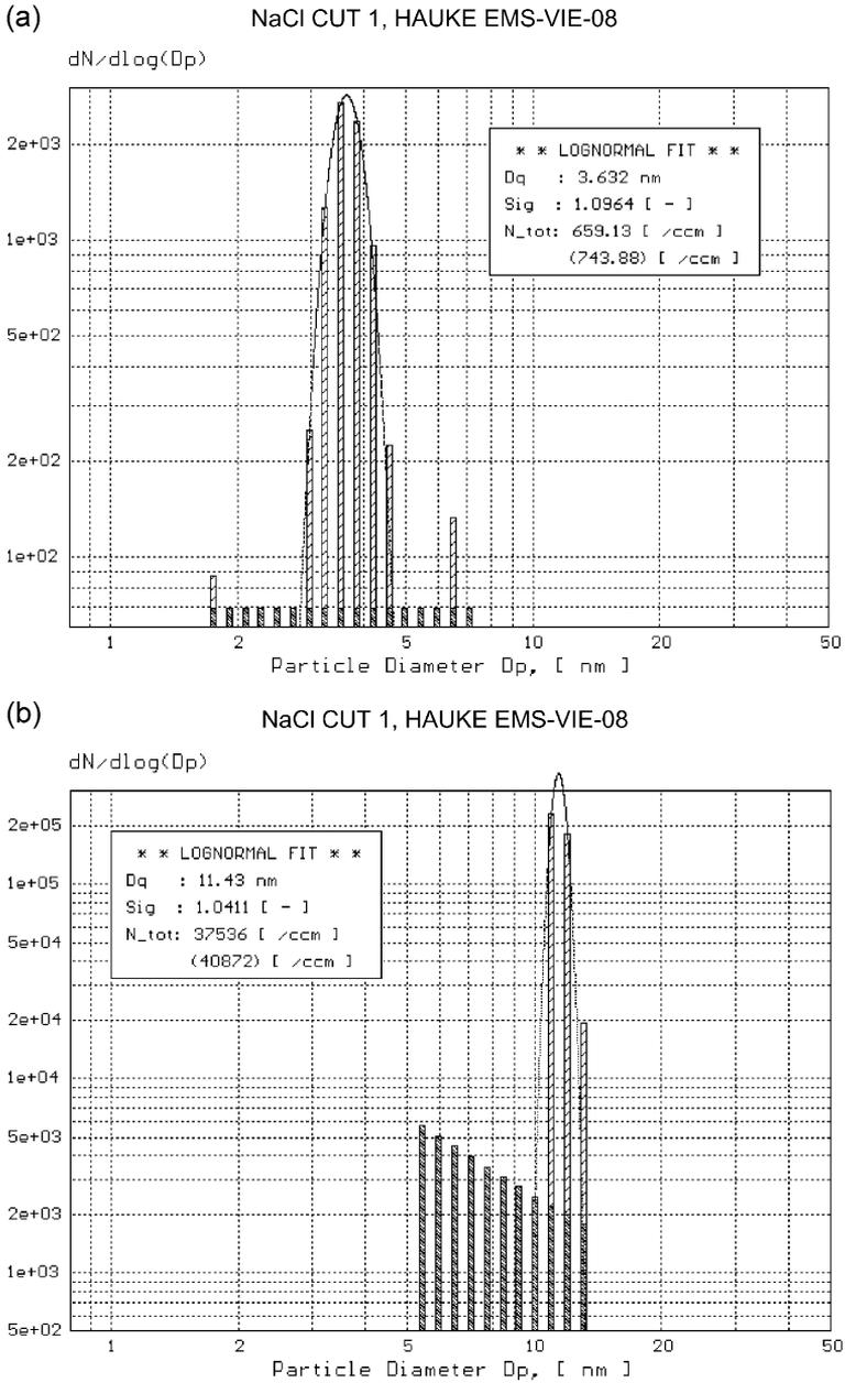
Fig. 2. Sample size distributions of monodispersed NaCl test aerosol, geometric mean particle diameter of 3.6 nm (a), 11.4 nm (b) and 18.5 nm (c), as measured by means of the HAUKE EMS-08.
