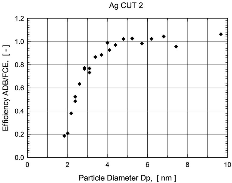
Fig. 10. Experiment Ag CUT 2: response characteristics of the readjusted automated diffusion battery (ADB) for monodispersed NaCl test aerosols, geometric mean particle diameters between 1.8 and 10 nm.
