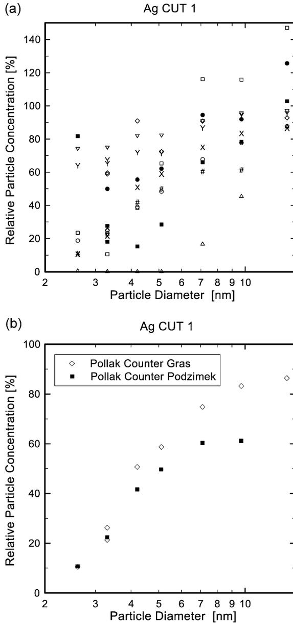
Fig. 9. Experiment Ag CUT 1: response characteristics of all participating instruments for monodispersed Ag test aerosols, geometric mean particle diameters between 2.5 and 20 nm (a), comparison of the performance of subsets of instruments, PCG and PCP (b) and the dibutyl phtalate operated instruments TM CNC, ADB and DAS (c).
