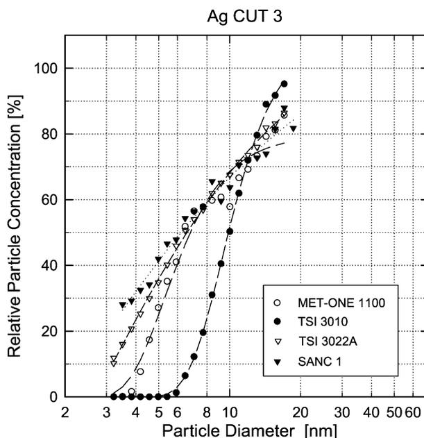
Fig. 11. Experiment Ag CUT 3: response characteristics of a subset of instruments (MET ONE-1100, TSI 3010, TSI 3022A and SANC I) for monodispersed Ag test aerosols, geometric mean particle diameters between 3 and 20 nm.
