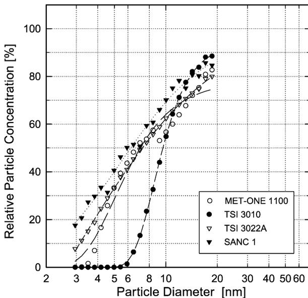
Fig. 13. Experiment Tungsten Oxide CUT 1: response characteristics of a subset of instruments (MET ONE-1100, TSI 3010, TSI 3022A and SANC I) for monodispersed tungsten oxide test aerosols, geometric mean particle diameters between 2.5 and 20 nm.
