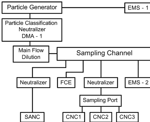
Fig. 1. Schematic diagram of the experimental arrangement showing the systems for aerosol generation, classification and dilution as well as the linear aerosol flow system and the various aerosol measurement instruments considered. The instruments used are listed in Table 1.
