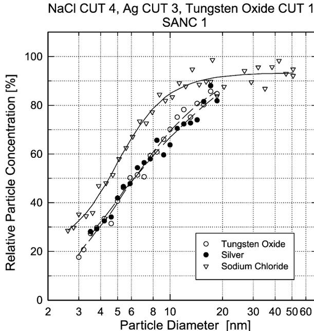
Fig. 19. Comparison of the response characteristics of the SANC I with respect to NaCl, Ag and tungsten oxide test aerosols.
