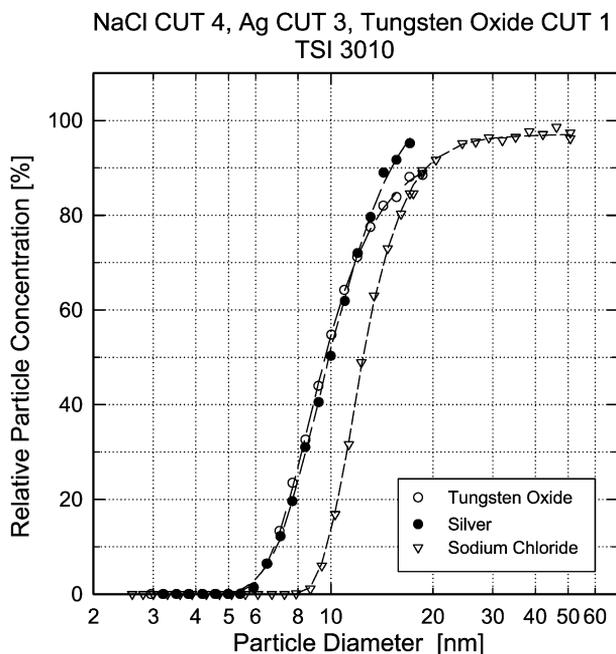
Fig. 17. Comparison of the response characteristics of the TSI 3010 condensation particle counter with respect to NaCl, Ag and tungsten oxide test aerosols.
