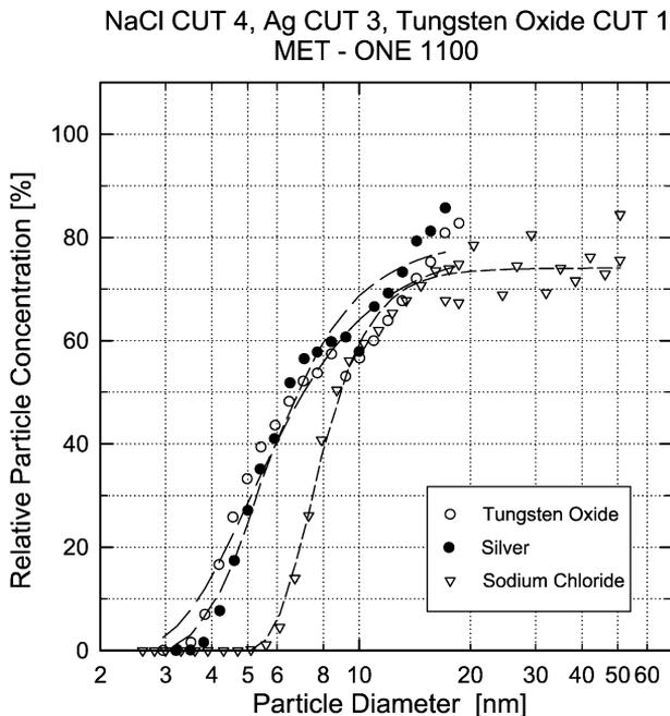
Fig. 16. Comparison of the response characteristics of the MET ONE-1100 condensation nucleus counter with respect to NaCl, Ag and tungsten oxide test aerosols.
