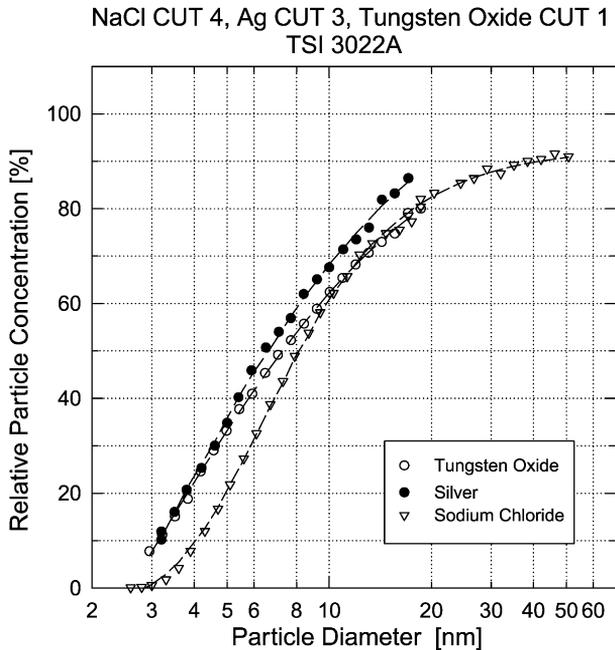
Fig. 18. Comparison of the response characteristics of the TSI 3022A condensation particle counter with respect to NaCl, Ag and tungsten oxide test aerosols.
