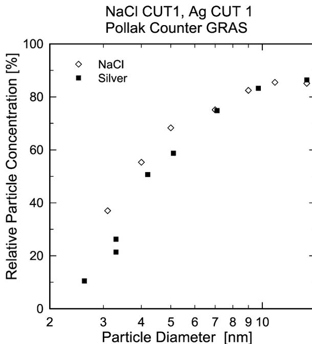
Fig. 15. Comparison of the response characteristics of the PCG Pollak counter with respect to NaCl and Ag test aerosols.
