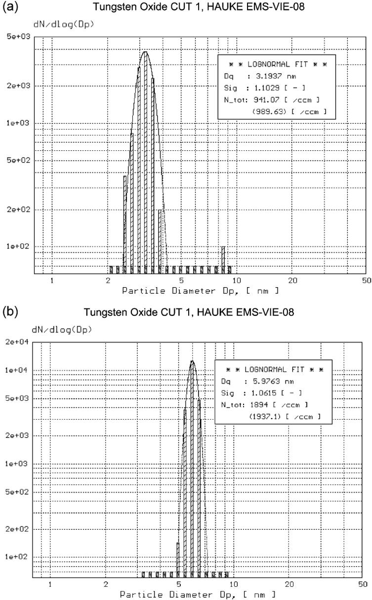
Fig. 12. Sample size distributions of monodispersed tungsten oxide test aerosols, geometric mean particle diameter of 3.2 nm (a), 6.0 nm (b) and 20.4 nm (c), as measured by means of the HAUKE EMS-08.
