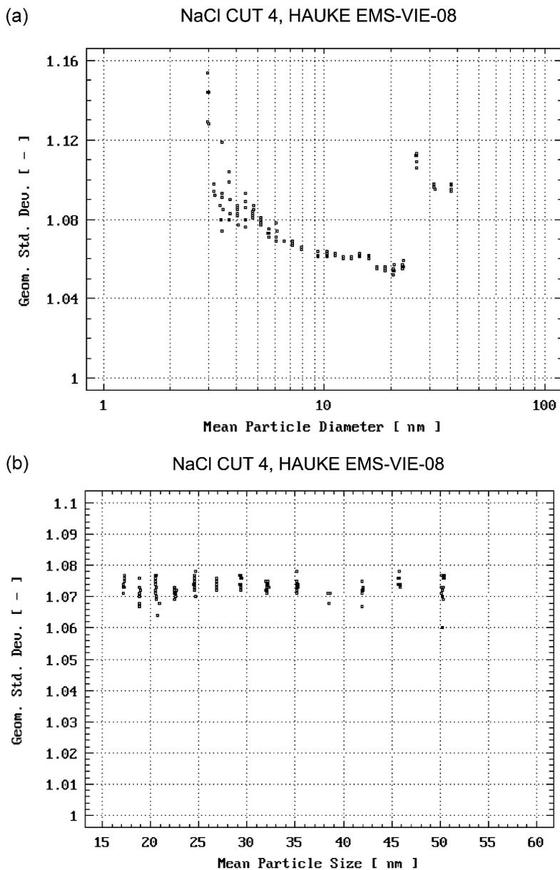
Fig. 6. Geometric standard deviations of NaCl test aerosols for the size range 3–20 nm (tube furnace generator with subsequent electrostatic classification) (a) and for 18–50 nm (collision atomizer with subsequent electrostatic classification) (b) used in experiment NaCl CUT 4.
