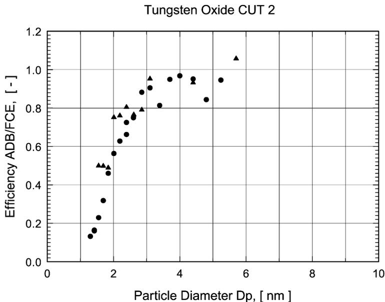
Fig. 14. Experiment Tungsten Oxide CUT 2: response characteristics of the readjusted automated diffusion battery (ADB) for monodispersed tungsten oxide test aerosols, geometric mean particle diameters between 1.5 and 6 nm.
