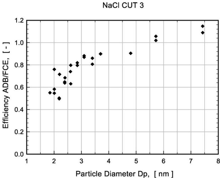
Fig. 5. Experiment NaCl CUT 3: response characteristics of the readjusted automated diffusion battery (ADB) for monodispersed NaCl test aerosols, geometric mean particle diameters between 1.8 and 8 nm.
