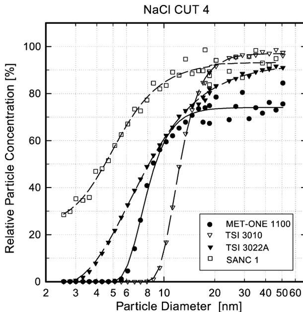
Fig. 7. Experiment NaCl CUT 4: response characteristics of a subset of instruments (MET ONE-1100, TSI 3010, TSI 3022A and SANC I) for monodispersed NaCl test aerosols, geometric mean particle diameters between 2.5 and 50 nm.
